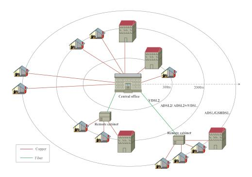
Figure 1.6 DSL technologies - distance vs. speed
