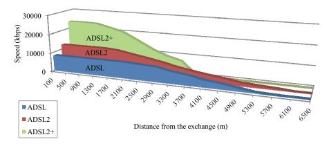
Figure 1.7 Characteristics of various ADSL technologies
